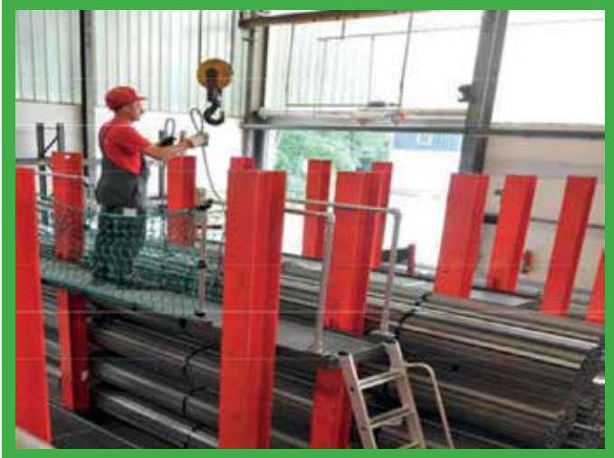
Safe access for attaching lifting hooks.
