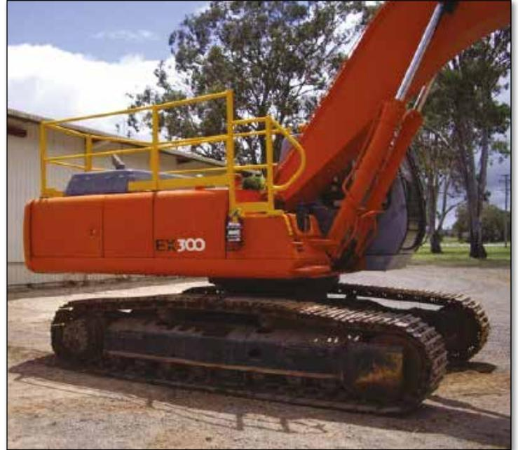
Safe Access: Note the handrails and access stairs and steps.
